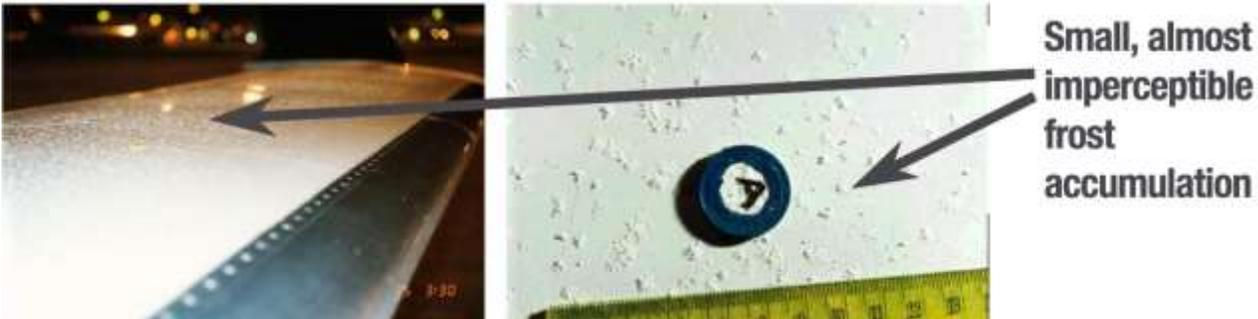
Frost can also reduce the max lift on our wings by up to 30%. Our Mooney wings are Laminar, so that could impact us more significantly.
