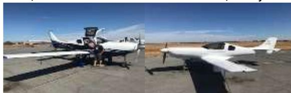
Lancair Planes at Paso, left is new four place "Mako", right is 2 place 320, both cruise at about 220K (250 MPH):
